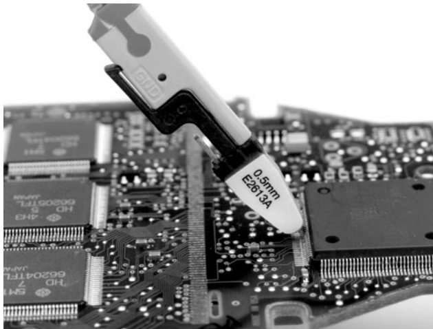
Easy hands-free connection to fine pitch ICs using the Wedge and 117x probe.
