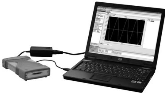
The U2300A data acquisition device setup in standalone operation.
