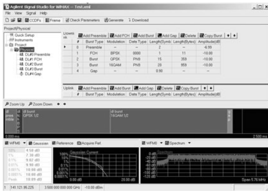
Summary of fixed WiMAX frame structure indicating burst types, modulation formats, data types, and more. Graphical plot of frame, CCDF curves, spectrum, and waveform spectrum.
