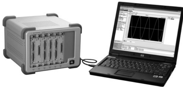
The U2300A data acquisition device setup in modular operation, with the U2781A chassis.
